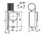
Thermostat with probe 380V - 15 A - IP40 capillary length 1 m contact NO (and NC)
