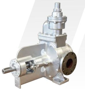
SRP-220 pump, shown set up for pumping asphalt, 200 GPM, at 150 PSI, 350°F. With high temperature paint and jacketed back cover for steam heating.
