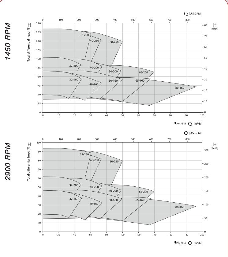
for handled Liquid with SG = 1000 kg/m<sup>3</sup>, Viscosity = MM<sup>2</sup>/s
